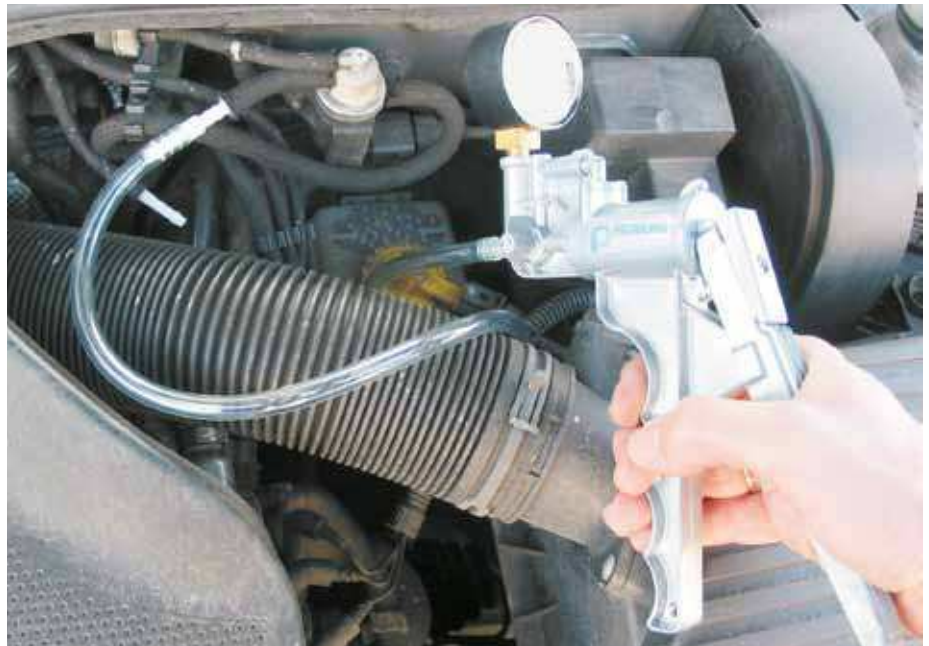
Checking an EPW using a manually operated vacuum pump (VW Golf IV)
